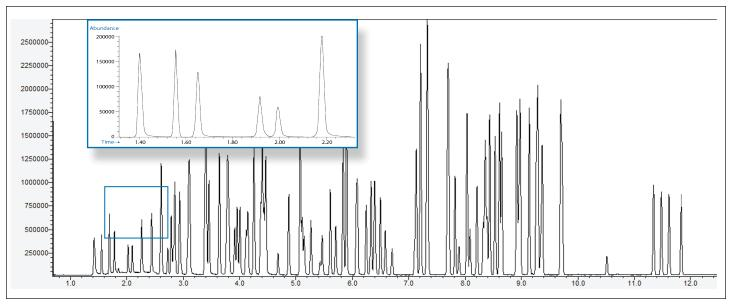
50 ppb EPA Method 8260. Front end gases showing improved resolution are highlighted.
