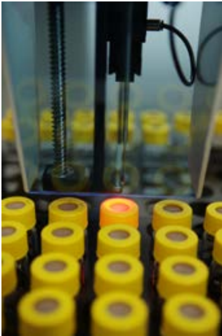
Fiber optic vial sensor eliminates lost vial error
