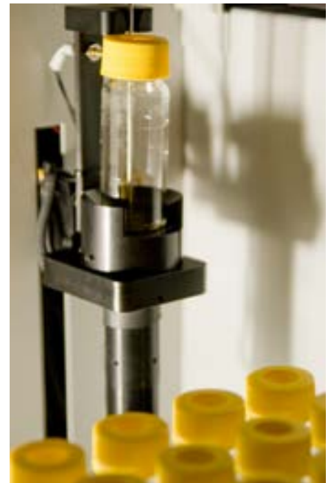
Samples run in the soil position can be heated and stirred while being purged
